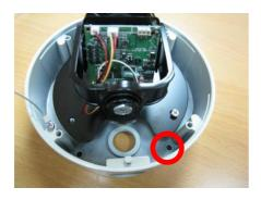
3. Tighten the 4 mounting screws to secure the camera body to the mounting surface.
